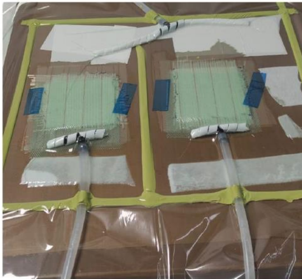
4 layers, 70^\circ\text{C} for 2h Porosity: < 2\% (ASTM D2734)
