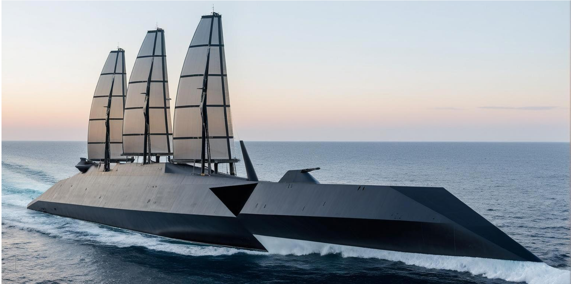
Example: 70m navy ship for hunting submarines with 3 Aero sail units
