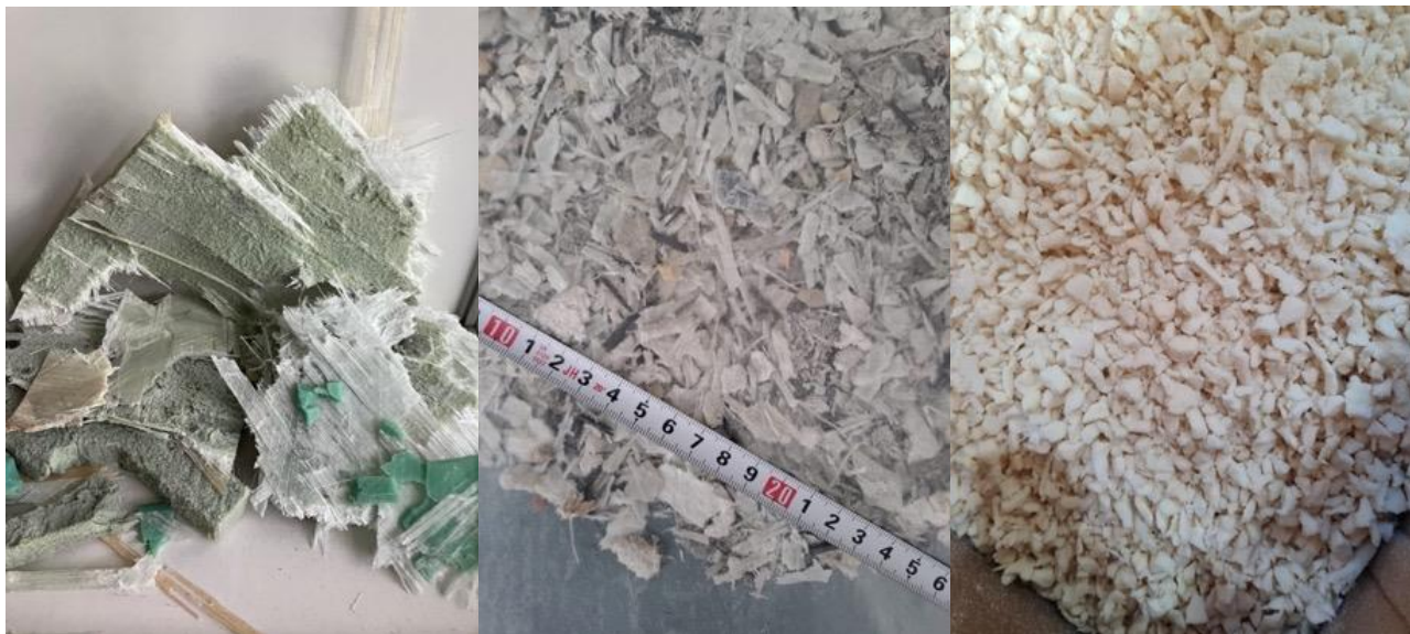
Figure 4 - Shredded and granulated blades - Gees Recycling
