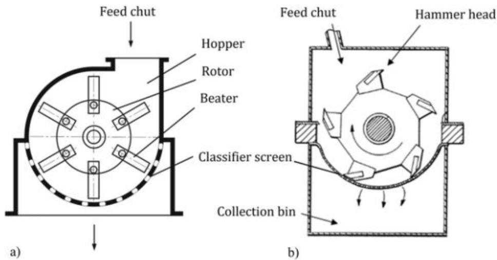
Figure 10: schematics of a rotating (a) hammer mill and (b) cutting mill, with changeable classifier screen. Taken from (Gonçalves et al., 2022), [CC BY 4.0](https://creativecommons.org/licenses/by/4.0/) license
