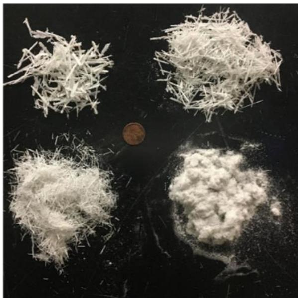
Figure 11: three stage classification of shredded GFRP. Taken from (Gonçalves et al., 2022), [CC BY 4.0](https://creativecommons.org/licenses/by/4.0/) license
