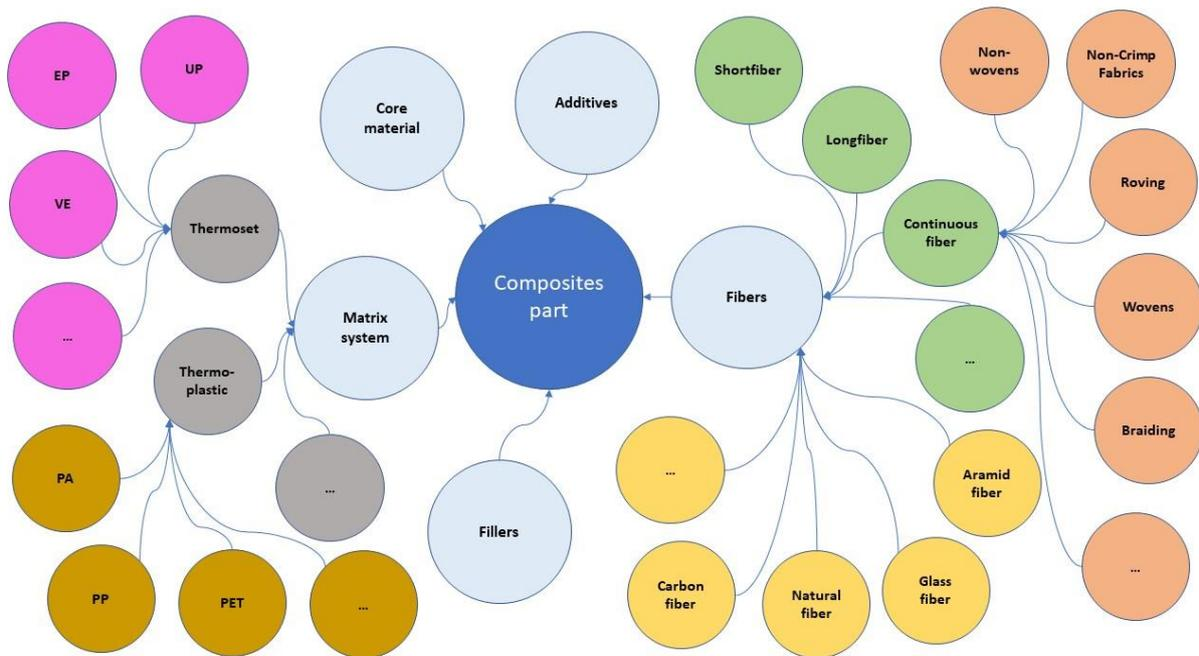
Figure 2: Exemplary input materials/combinations of composites
