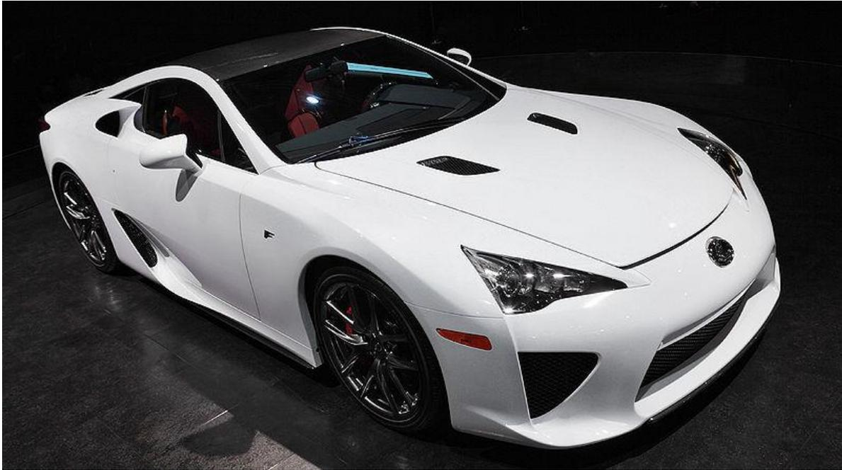
*Figure 31: example of a Lexus LFA. Its entire body was made of CFRP; 65% of this material was used in its construction, which saved up to 220 lbs (100 kg) and increased the rigidity of the whole vehicle. Taken from [Wikimedia Commons](#), [CC BY-SA 3.0](#) license*
