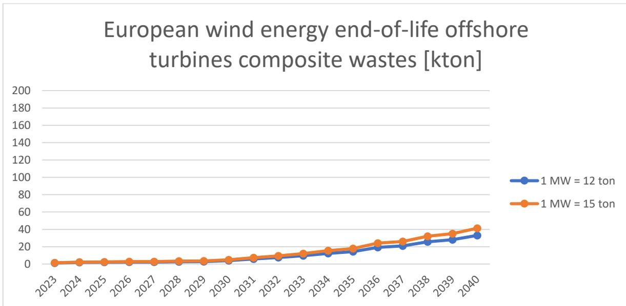
Figure 23: European wind energy end-of-life offshore turbines composite wastes
