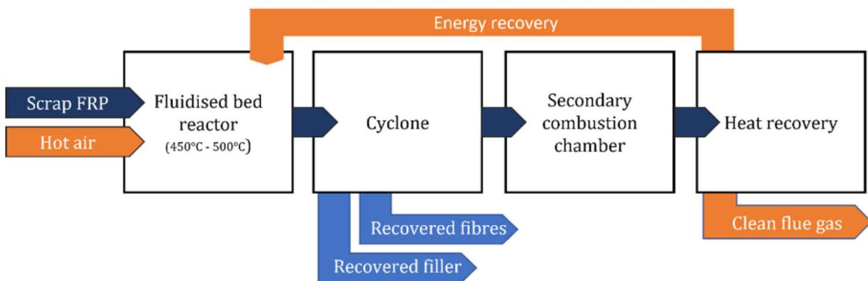
Figure 13: fluidized-bed recycling process. Taken from (Gonçalves et al., 2022), [CC BY 4.0 license](#)
