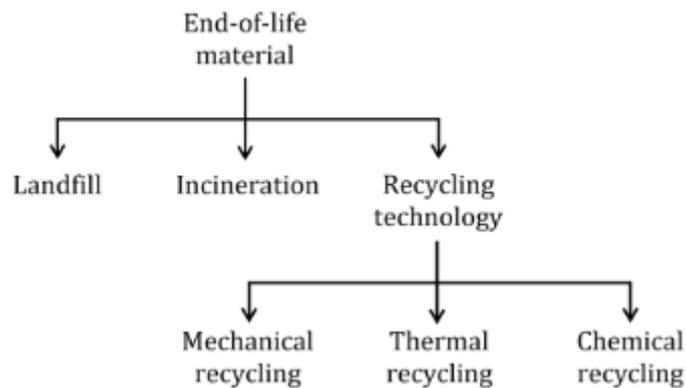
Figure 9: Representation of different recycling processes for thermoset composite materials. Simplified from (Gonçalves et al., 2022), [CC BY 4.0 license](#)
