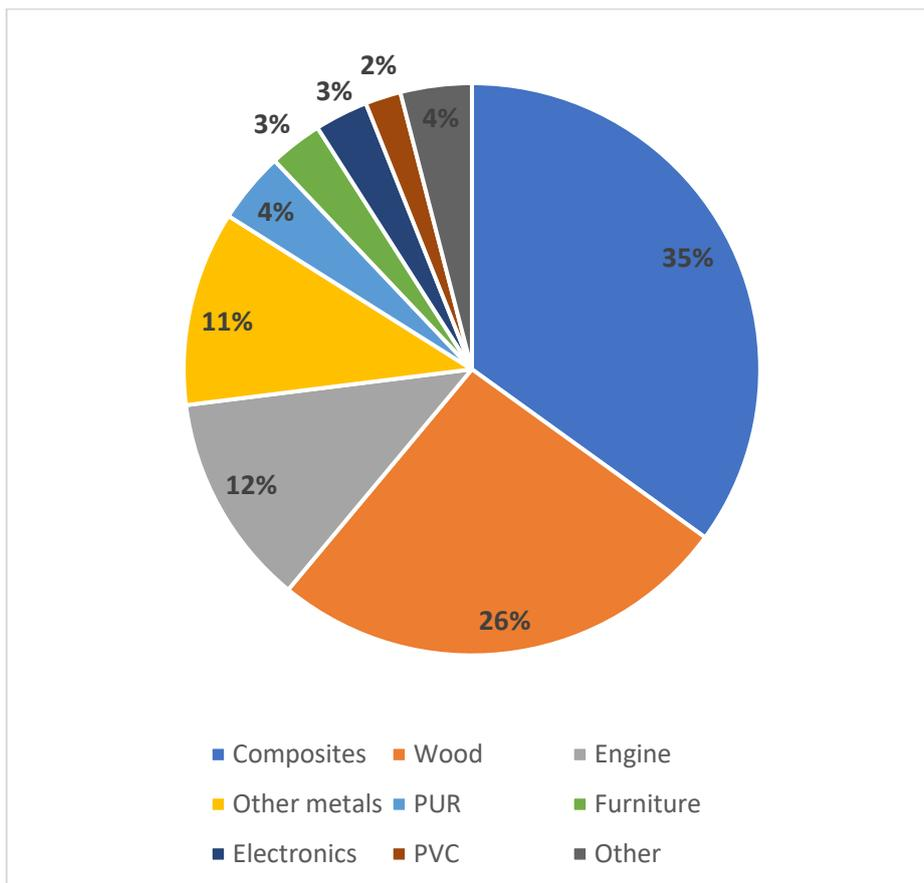
Figure 28: detailed material composition for a Selco queen 24 feet (Eklund et al., 2013)
