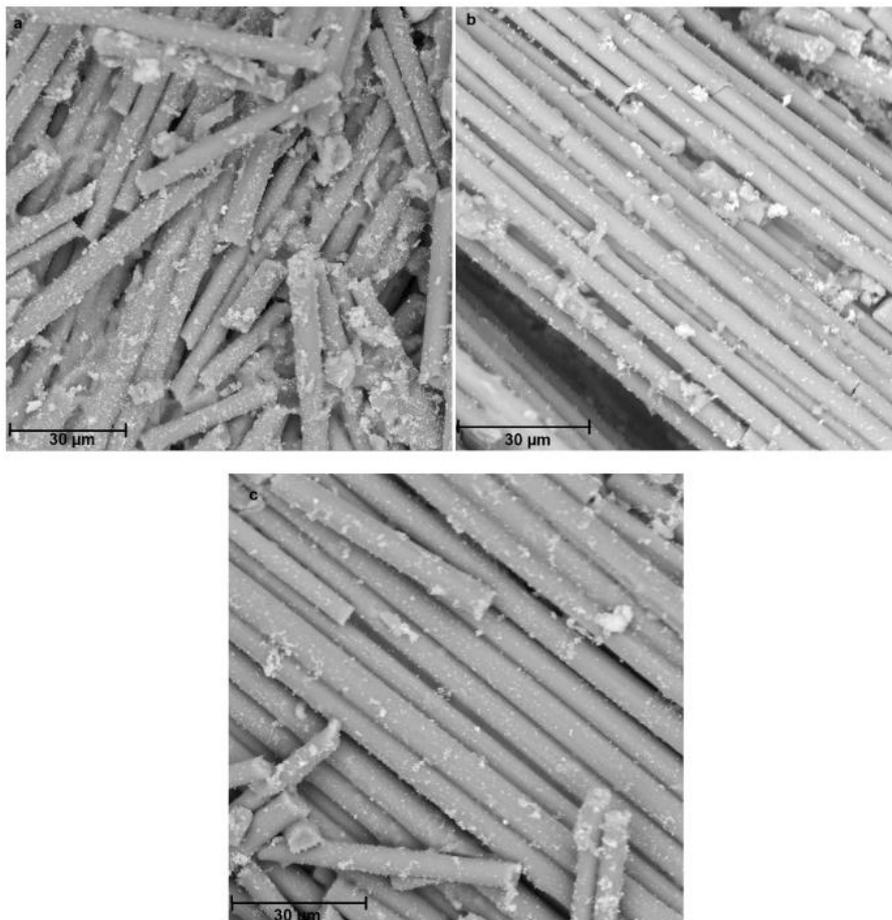
Figure 12: SEM images of carbon fibers after pyrolysis. (a) 480 °C, (b) 520 °C, (c) 560 °C. Taken from (Schwarz et al., 2020), [CC BY 4.0 license](#)
