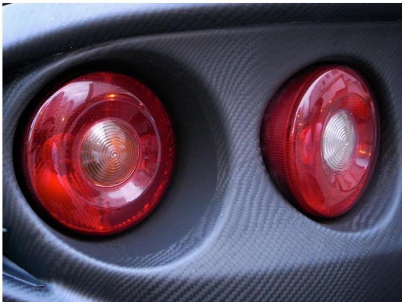
Figure 32: detail of a CFRP backlight frame. Taken from [Flickr](#), [CC BY-NC-ND 2.0](#) license
