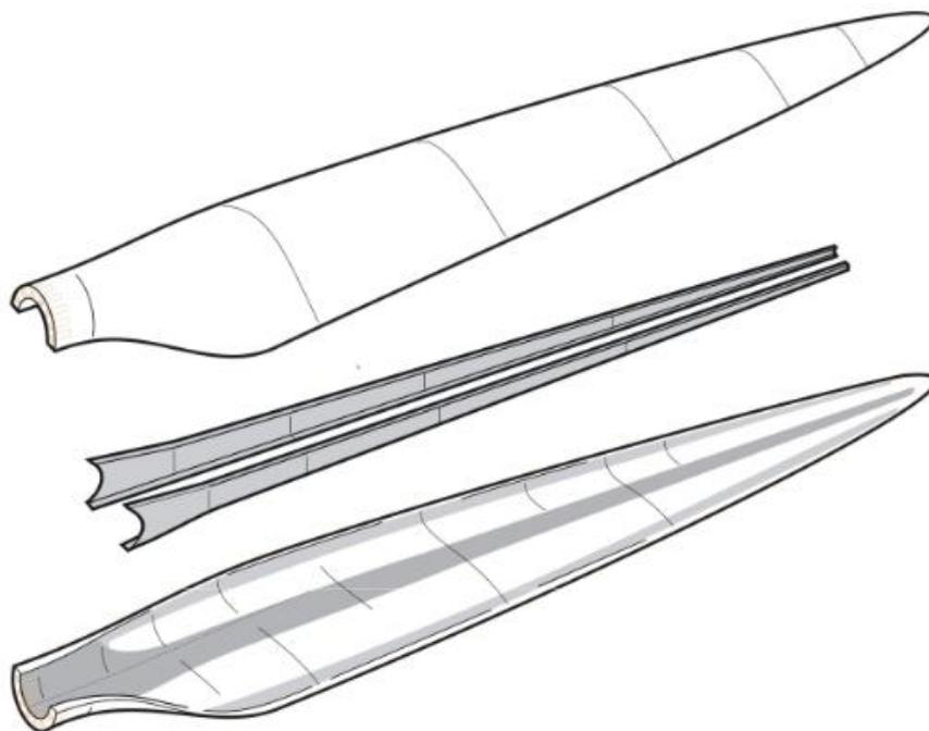
Figure 17: schematic longitudinal exploded view of a wind blade. Taken from (Mishnaevsky et al., 2017), [CC BY 4.0 license](#)
