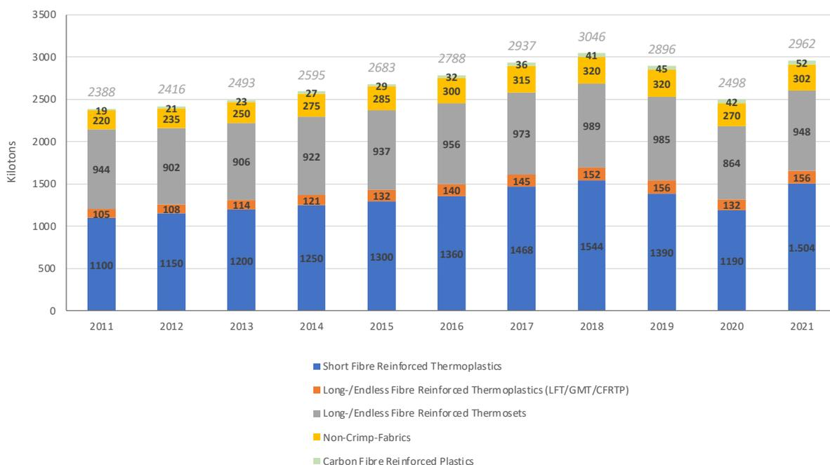
Figure 5: Composites production volume in Europe since 2011 (in 000 t) - Not included: Natural Fiber Reinforced Plastics (2012 = 90,000 tons) (AVK – Industrievereinigung Verstärkte Kunststoffe, 2021)
