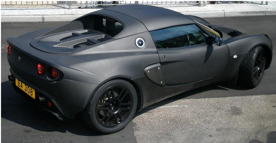
Figure 33: CFRP based Lotus Elise. Taken from [Flickr](#), [CC BY-NC-ND 2.0](#) license
